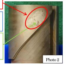
Photo 1 and 2 show the cases of actual cavitation erosion.
